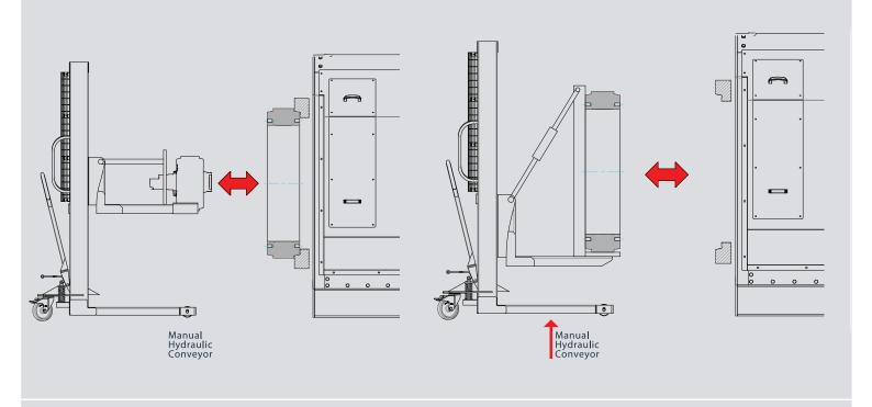
**The manual hydraulic stacker** facilitates die and roller installation. It delivers die and rollers to the storage area, removing the need for any further operations.
