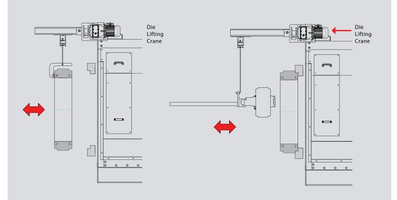
It is a **motorized mechanical crane system** that enables the easy lowering and lifting of the die and rollers. The crane is specifically anchored on the pellet mill. It works with up-down commands over the hand control.
